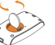
2. Install the battery with "+" side upward and keep it under the metal connector.
